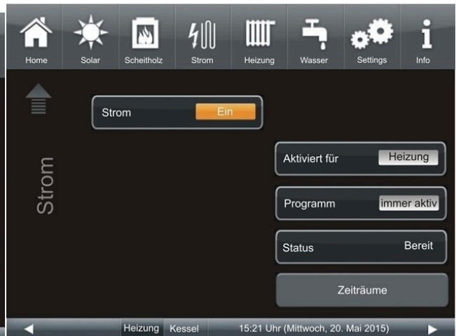
Illustration 5: Auxiliary heater 2 side 2: with electricity (= Strom) (electric heating element without power measurement option)
