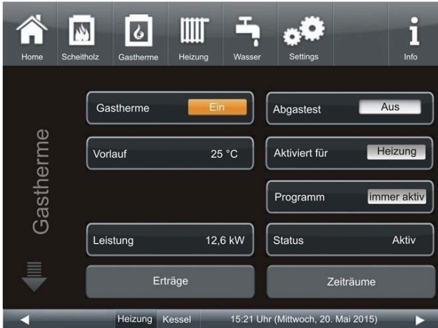
Illustration 3: Auxiliary heating 1 (=ZH) menu (1st page) with EWP output for gas boiler (ZH 1) with display of output and flow temperature
