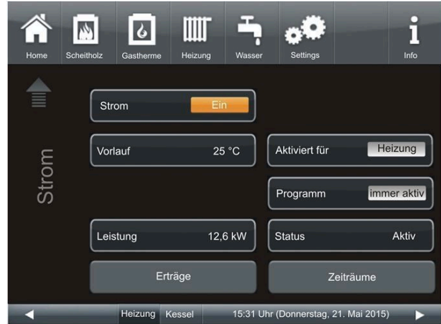
Illustration 4: Auxiliary heating 2 (=ZH) menu (2nd page) with EWP output for electric heating (ZH 2)
