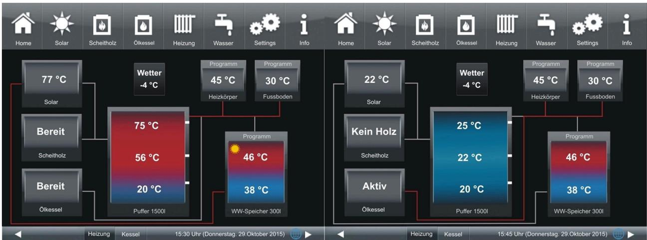
*Illustration 3: EWP oil-gas-solar; solar loading for hot water cylinder. Heating circuit charging via system cylinder*
