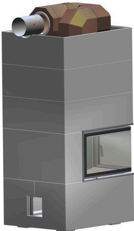
Im. 20: Place second level MSS and second top ring
