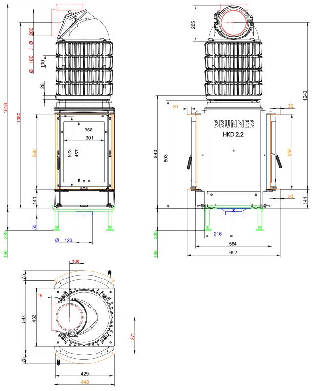
...round with door frame and Heat exchanger rings
