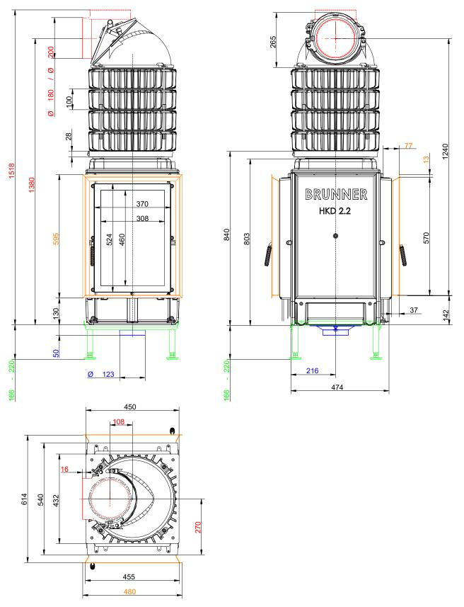
... flat with door frame and Heat exchanger rings
