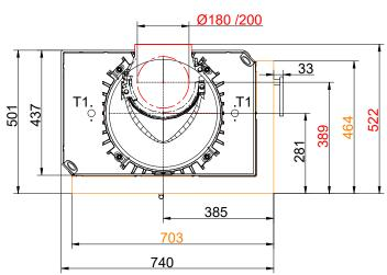
... right with mounting bracket and cast iron heat exchanger rings + dome (side-opening door, DT)
