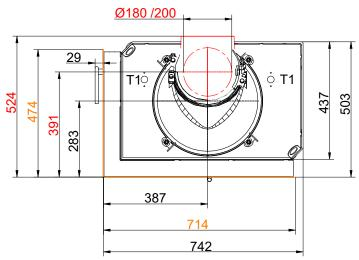
... left with door frame and cast iron dome (side-opening door, DT)
