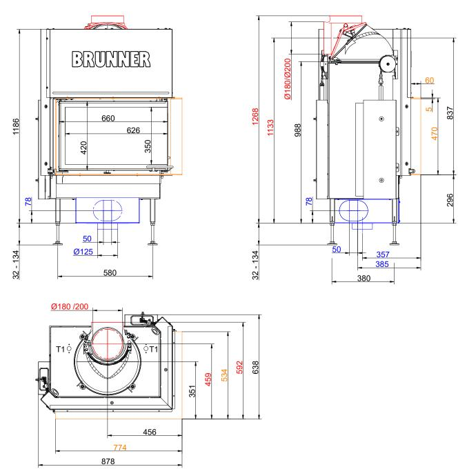
... right with mounting frame and cast iron dome (lifting door, ST)
