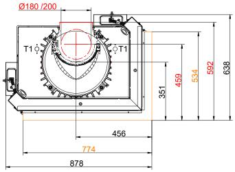
... right with mounting frame and cast iron heat exchanger rings + dome (lifting door, ST)
