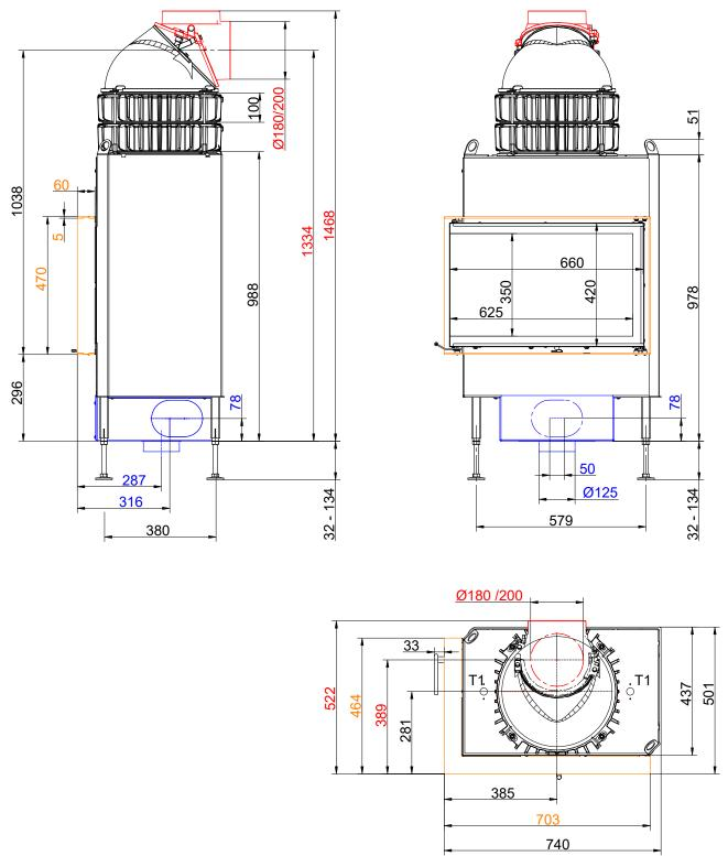
... left with mounting bracket and cast iron heat exchanger rings + dome (side-opening door, DT)
