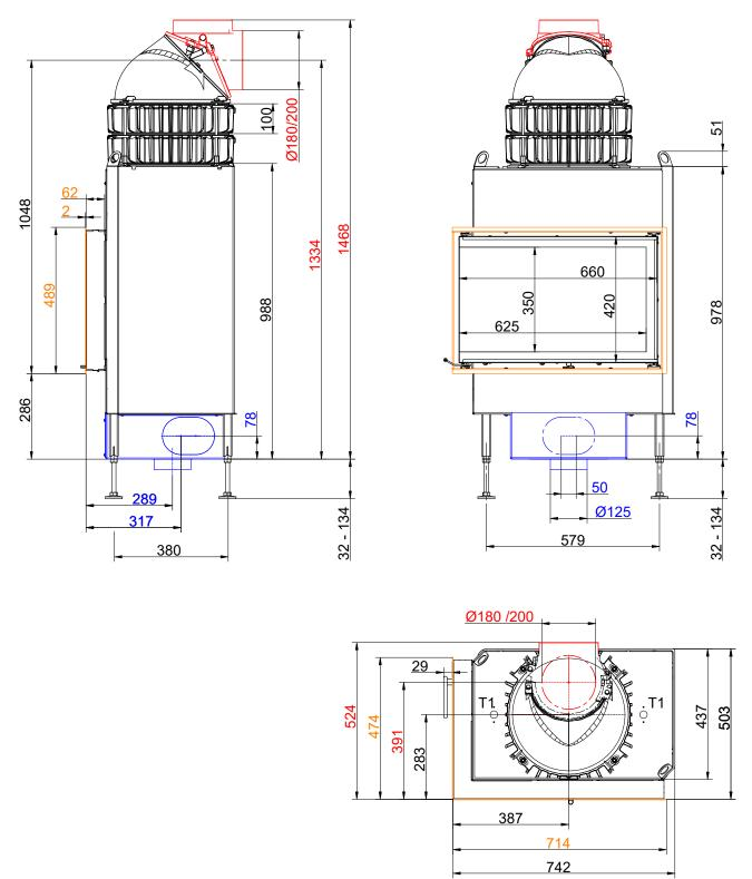
... left with door frame and cast iron heat exchanger rings + dome (side-opening door, DT)
