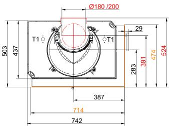
... right with door frame and cast iron dome (side-opening door, DT)
