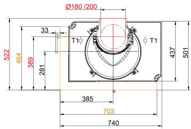
... left with mounting bracket and cast iron dome (side-opening door, DT)
