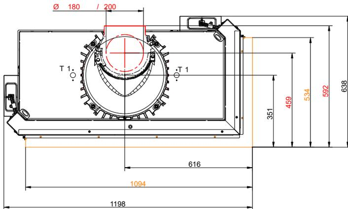
... right with mounting frame and cast iron heat exchanger rings + dome
