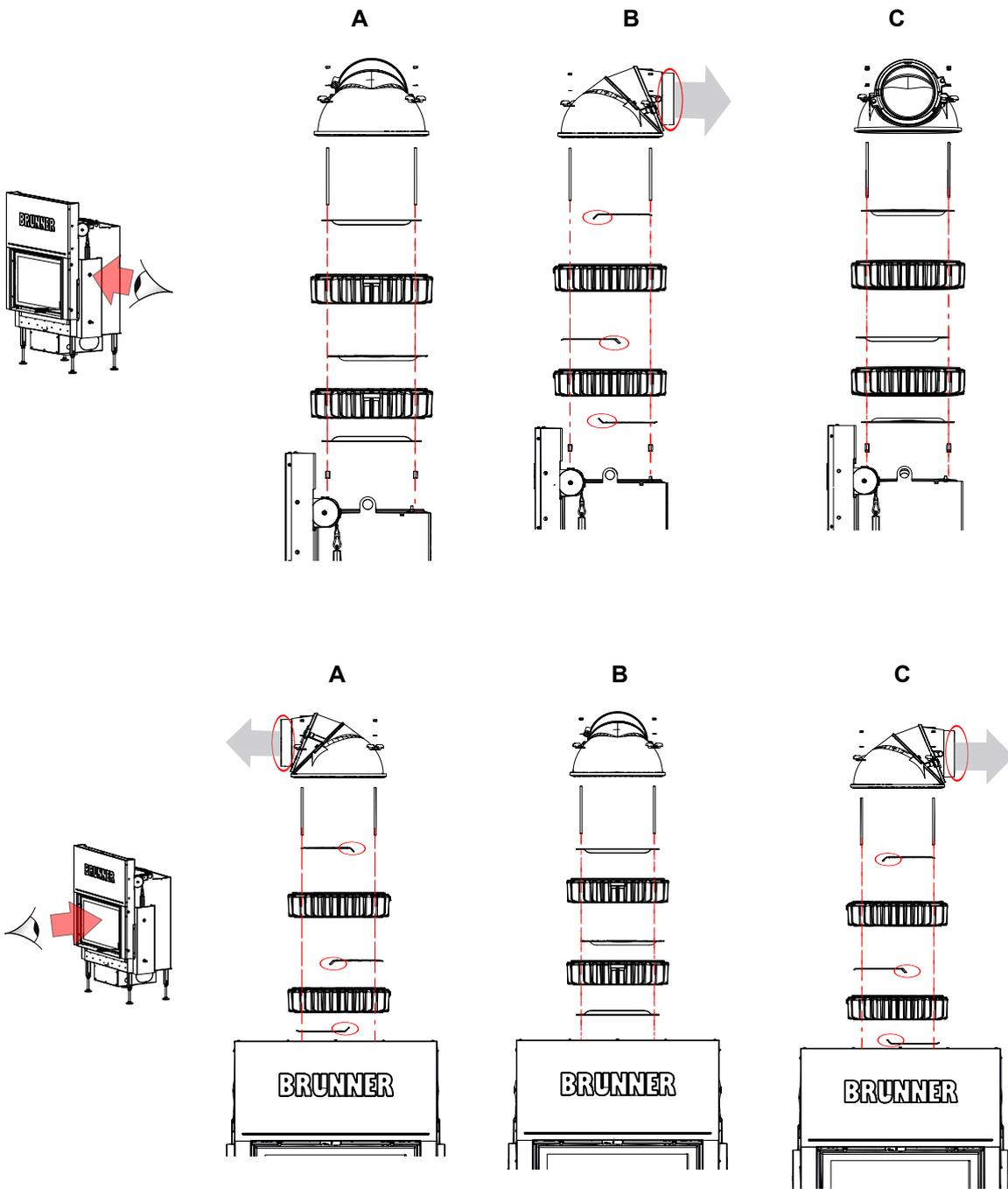
5) Example F: with rotating cast iron dome with cast iron heat exchanger rings - to the left vertical or horizontal
