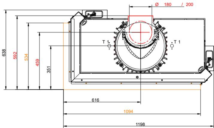
... left with mounting frame and cast iron heat exchanger rings + dome
