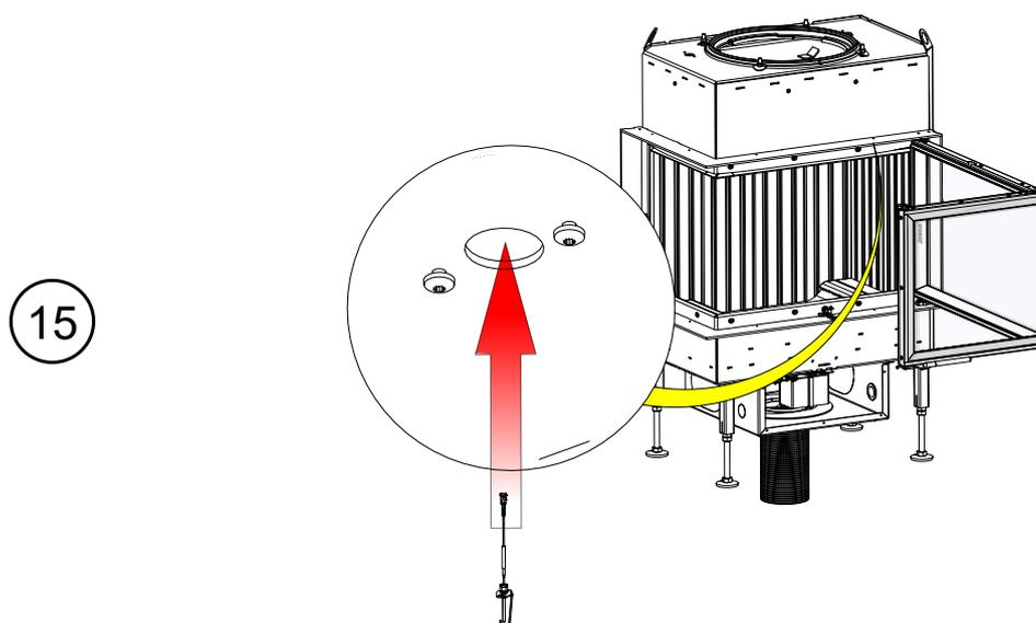
**i** Do not overtighten the screws!
