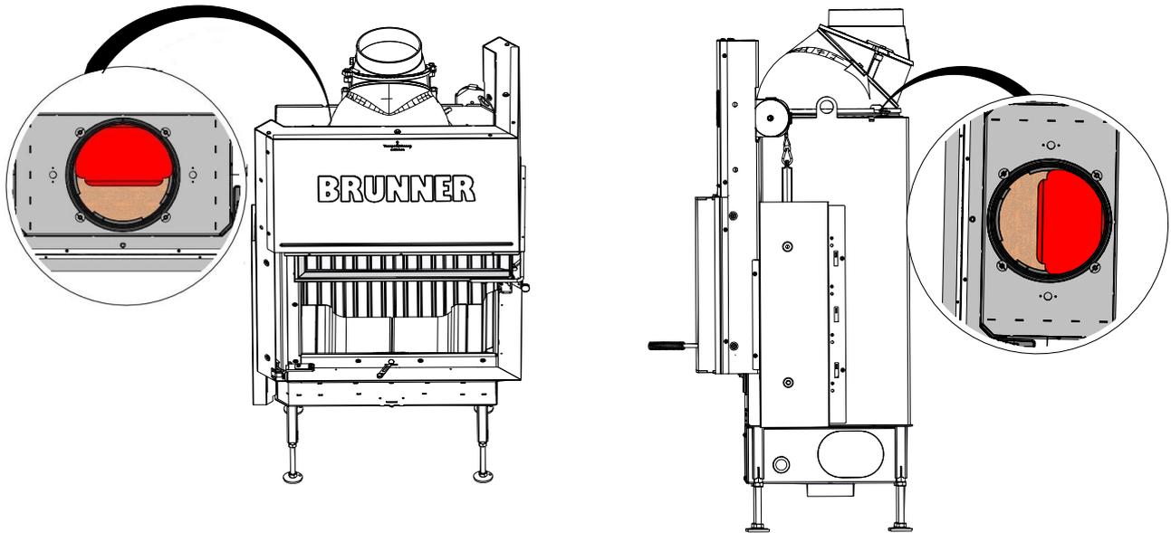
2) Example B: with rotating cast iron dome - at rear - horizontal
