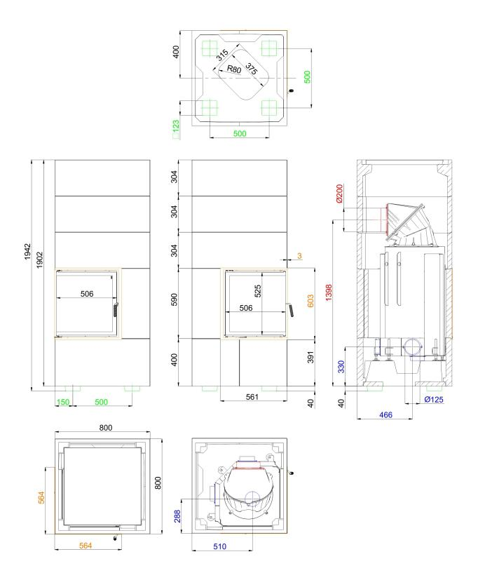
... with side opening door (frame (orange), combustion air nozzle (blue), levelling feet (green) marked in color)
