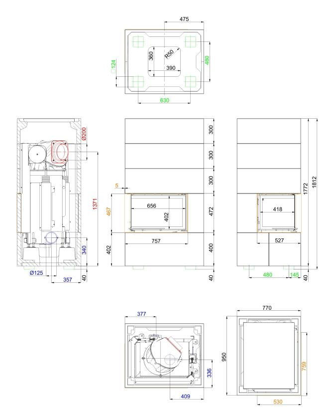
... left (frame (orange), combustion air nozzle (blue), levelling feet (green) marked in color)
