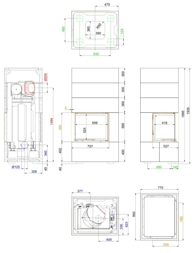
... left (frame (orange), combustion air nozzle (blue), levelling feet (green) marked in color)
