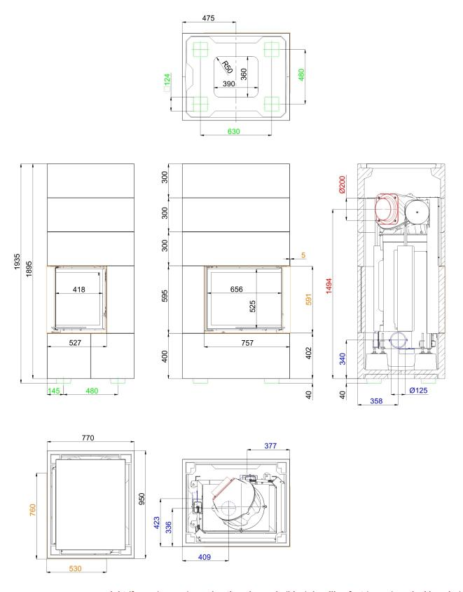
... right (frame (orange), combustion air nozzle (blue), levelling feet (green) marked in color)
