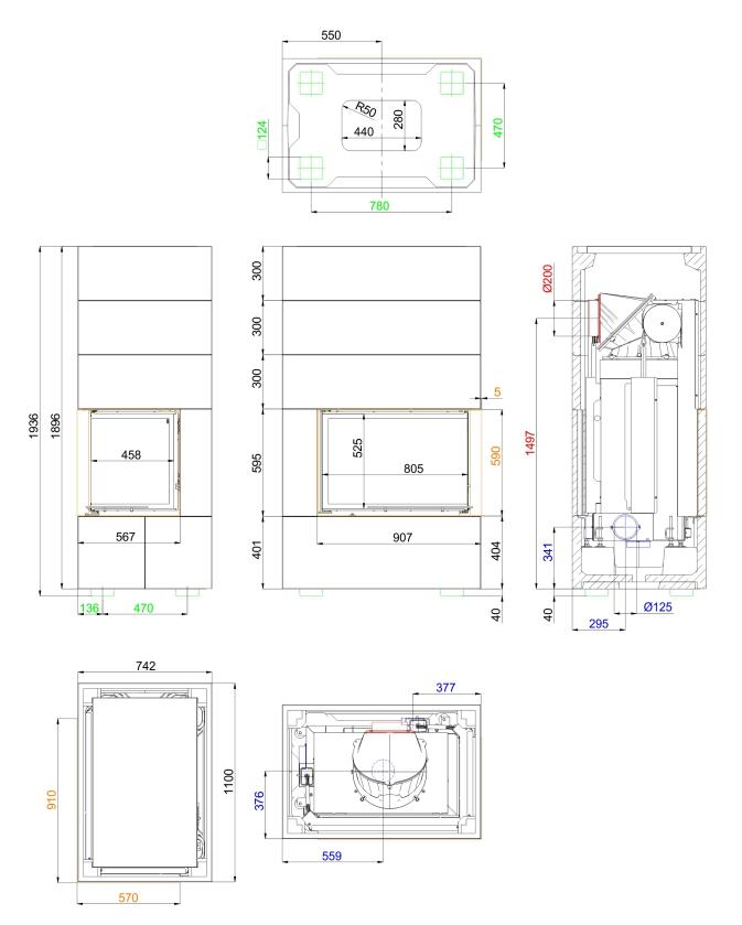
... right (frame (orange), combustion air nozzle (blue), levelling feet (green) marked in color)
