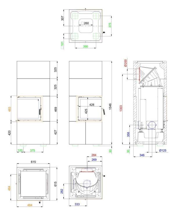
... cast iron hot air hood (frame (orange), combustion air nozzle (blue), levelling feet (green) marked in color)
