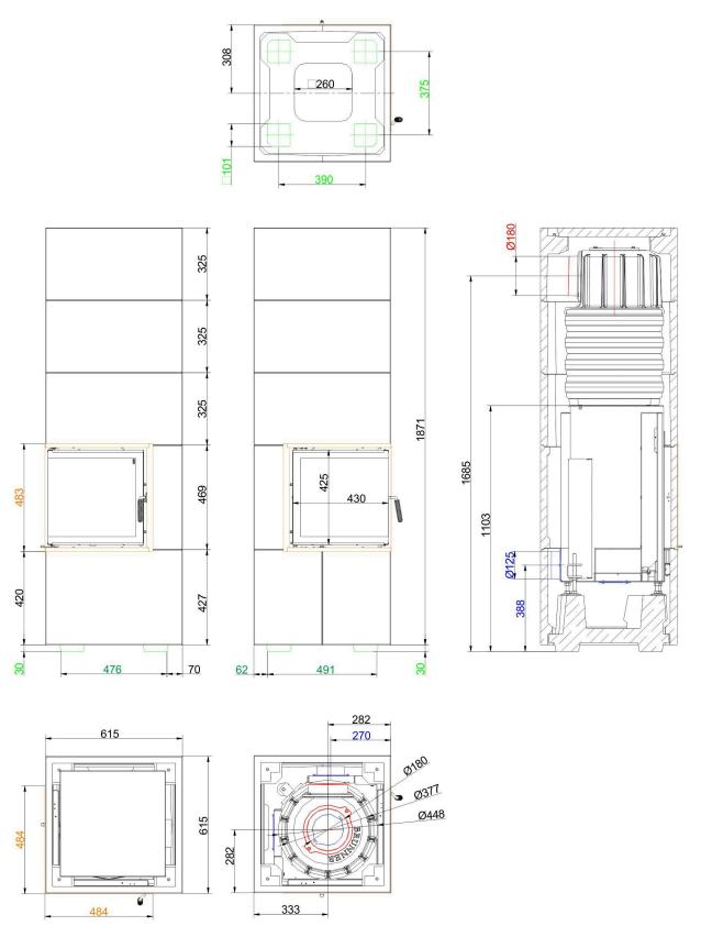
... with MAS (frame (orange), combustion air nozzle (blue), levelling feet (green) marked in color)
