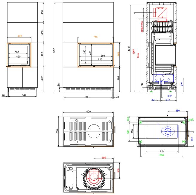
... right, frame (orange), combustion air nozzle (blue), levelling feet (green)
