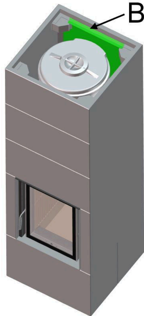
Im. 6: Installation position of the radiation protection plates (B)
