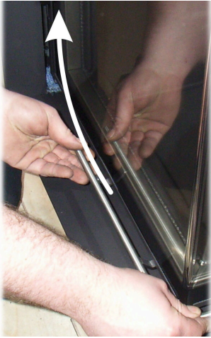
Illustration 4: Closing the door left side
