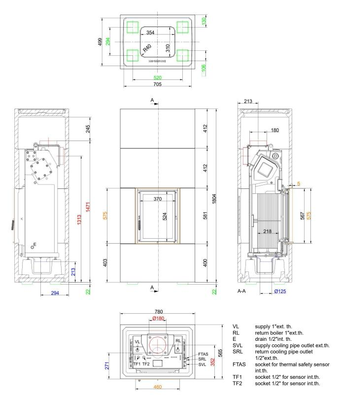
frame (orange), combustion air nozzle (blue), levelling feet (green) marked in color
